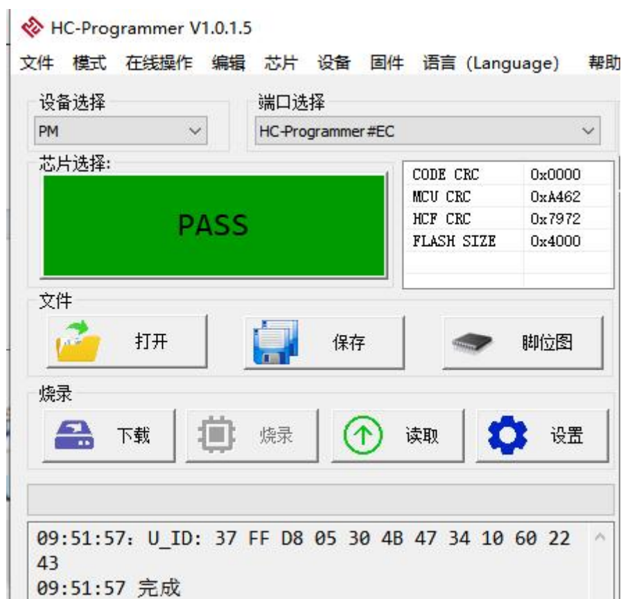
图 3.2.6-2 查询设备 UID
