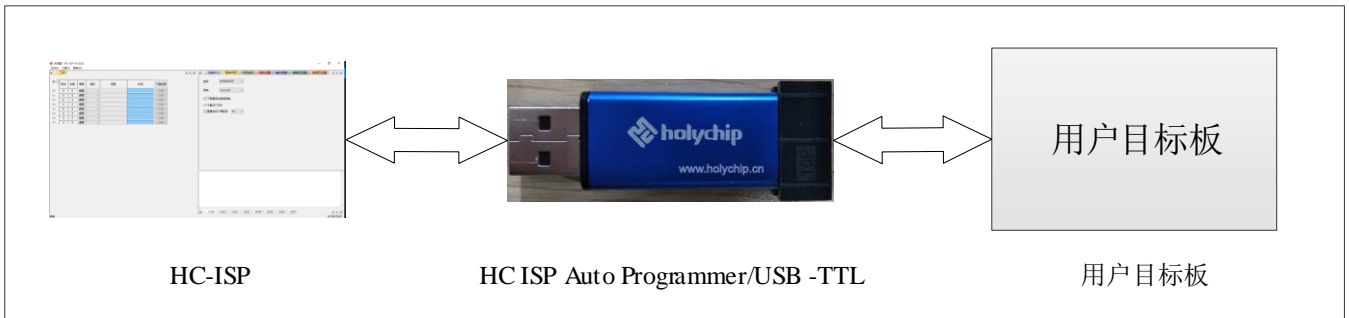
Figure 2-1 硬件连接(HC ISP Auto Programmer)
